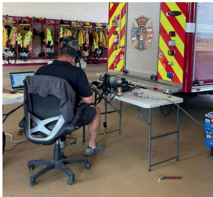
RFD completed annual SCBA flow testing per the NFPA Standard.
