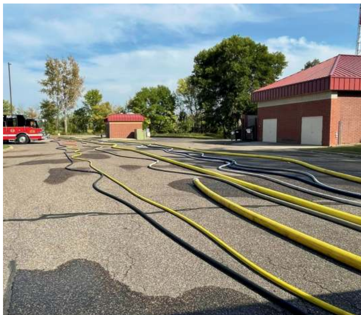
RFD completed annual hose test per the NFPA Standard.
