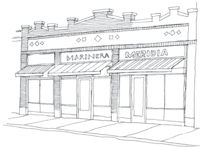
Rehabilitation of the same building, including uncovering of window, restoration of sign panels, and installation of awnings. Illustration: Robert Roscoe, Design for Preservation and City of Minneapolis.
