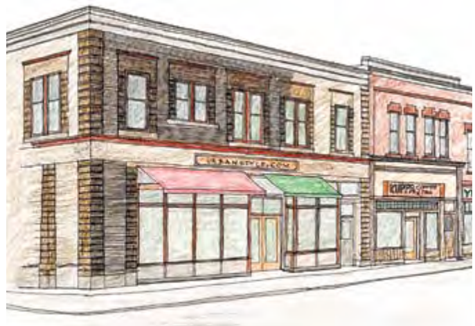
Rehabilitation of the same building, including removal of wood panels, tuckpointing of brick, uncovering of transom windows, restoration of sign panels, and installation of awnings. Illustration: Robert Roscoe, Design for Preservation and City of Minneapolis.
